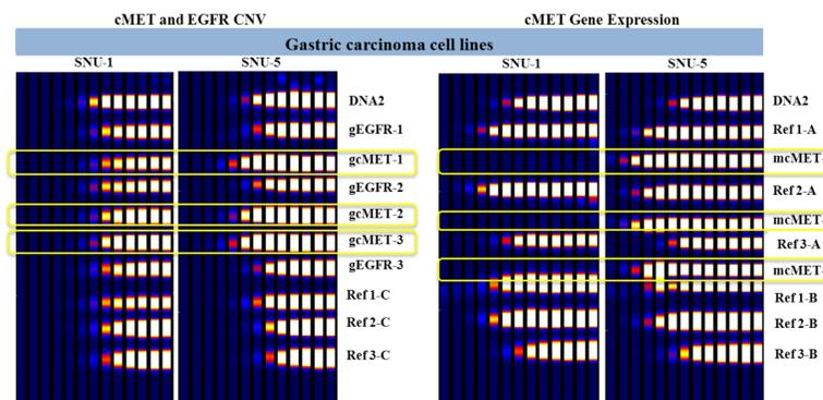
Figure 3. Representative electropherograms of cMET/EGFR CNV and cMET Gene Expression Assay generated on the ICEPlex System.
