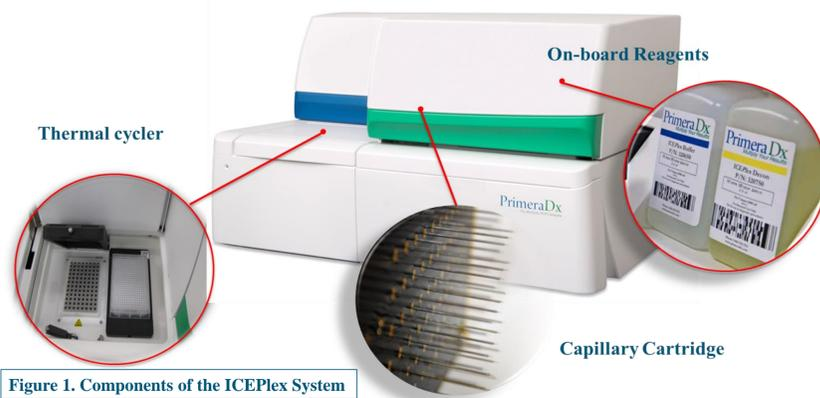
Figure 1. Components of the ICEPlex System
